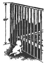
Guidelines recommend eliminating handholds and footholds and minimizing the size of openings in a barrier's construction. For a Solid Barrier:
