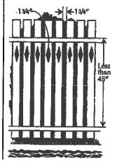
If the distance between the tops of the horizontal members is more than 45 inches, the horizontal members can be on the side of the fence facing away from the pool. The spacing between vertical members should not exceed 4 inches. This size is based on the head breadth and chest depth of a young child and is intended to prevent a child from passing through an opening. Again, if there are any decorative cutouts in the fence, the space within the cutouts should not exceed 1-3/4 inches.
